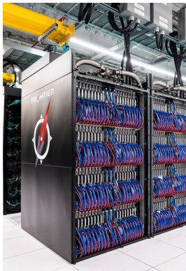
Figure: Frontier, the first exascale supercomputer in the United States. Credit: OLCF, Wikimedia Commons CC2.0.
